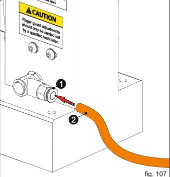
Install the hose coming from your compressor to the main air entrance of the machine (fig. 100). Then by starting the machine, test whether the adjusted height is proper for your project. If not, readjust the height by following the instructions in the previous step. Once the adjustment is made properly, tighten the nut of the adaptor and keep using the machine.
