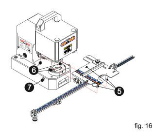
Remove the fixing screw from the machine. Place the pins for CSGSP-1 for on the holes for CS-TIDY-51 and tighten the fixing screw for as shown in (fig. 17).
