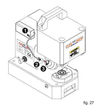
Locate the battery box 2 to the pre cleaned area 1 and keep pushing it to the machine for around 15 seconds to securely adhere it.
