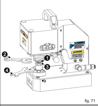
Place the wrenches ②, ④ that come with the machine on upper die adaptor ⑤ and its nut ⑥. By keeping the wrench ⑥ on the upper die adaptor still, loosen the nut ⑥ by rotating the other wrench ②. Then rotate the upper die adaptor ⑥ with the wrench ⑥ to adjust the required height.
