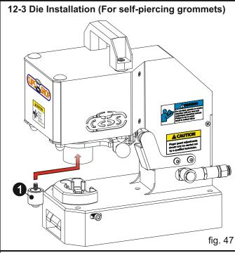
Locate the upper die **1** to the upper die holder/shaft center\* manually.
