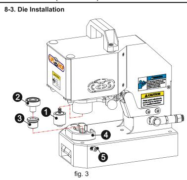
Important Note: 1) Be sure that the upper die adaptor is securely fixed to the shaft and the upper die is securely fixed to the die adaptor at all times. During a production run check that the upper die has not loosened from the die adaptor. Using the machine with a loose upper die can damage the threads of the die and the die adapter.
