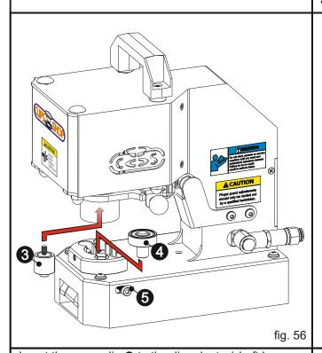
Insert the upper die **3** to the die adaptor/shaft by rotating manually or with a suitable wrench as shown in (fig. 56). Insert the lower die **4** into the lower die holder and secure its position by tightening the screw **5** with a screwdriver.
