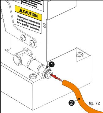
Install the hose coming from your compressor to the main air entrance of the machine. Then by starting the machine, test whether the adjusted height is proper for your project. If not, readjust the height by following the instructions in the previous step. Once the adjustment is made properly, tighten the nut of the adaptor and keep using the machine.
