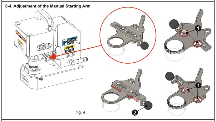
In order to avoid any damage during transportation, the manual starting arm of the machine is set to tightest position in factory settings. This arm is needed to be extended by the user for proper use. Loosen the wing nuts manually. Pull the manual starting arm in the arrow direction and adjust the length of it. Then securely fix the wing nuts manually as shown in (fig. 4).
