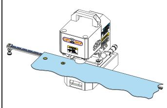
Lean your material's edge to the edge guide 3. Attach the first grommet. Poke this grommet through the grommet holder . Recline your material to the edge guide by sliding it as shown in the figure in arrow direction. Repeat these steps on the subsequent grommets you will attach.
