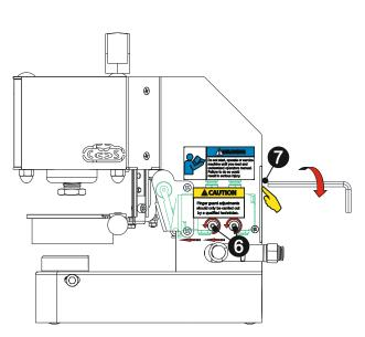
Pull down the manual start arm slowly. Though the acrylic safety guard gets closer than 6 mm to the lower die holder, if the die adapter does not move down, then follow the procedures illustrated in (fig. 64) after double checking the machine is connected to air source and there is pressurized air in the system.
