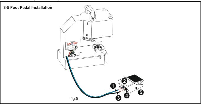
To avoid any damage during transportation, foot pedal **9** is packed unassembled in the factory and needs to be installed by the user.
