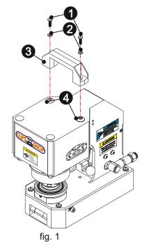
Poke the bolts through the washers then the hole of the handle and fix them to the bolts with threaded head by using a screwdriver as shown in (fig. 1).
