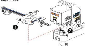
**Important Note:** Lower die should be attached and fixed before the installation of CSGSP-2. With use of #7.5 and bigger size dies, CSGSP-2 is installed directly to the lower die. For #5.5 and smaller sizes, CSGSP-2 should be mounted to the lower die holder. "Lower die holder" should be read as "Lower Die" in case it is used with #7.5 and bigger size dies in the following explanations.
