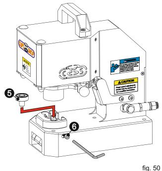
Depending on the type of die set you would like to install, insert the lower die into the the die bush or into the lower die holder. Fix the lower die by tightening the screw with a allen key.
