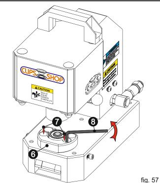
Loosen the fixing Allen screws **②** located inside the lower die holder **③** with a suitable Allen wrench **③**.
