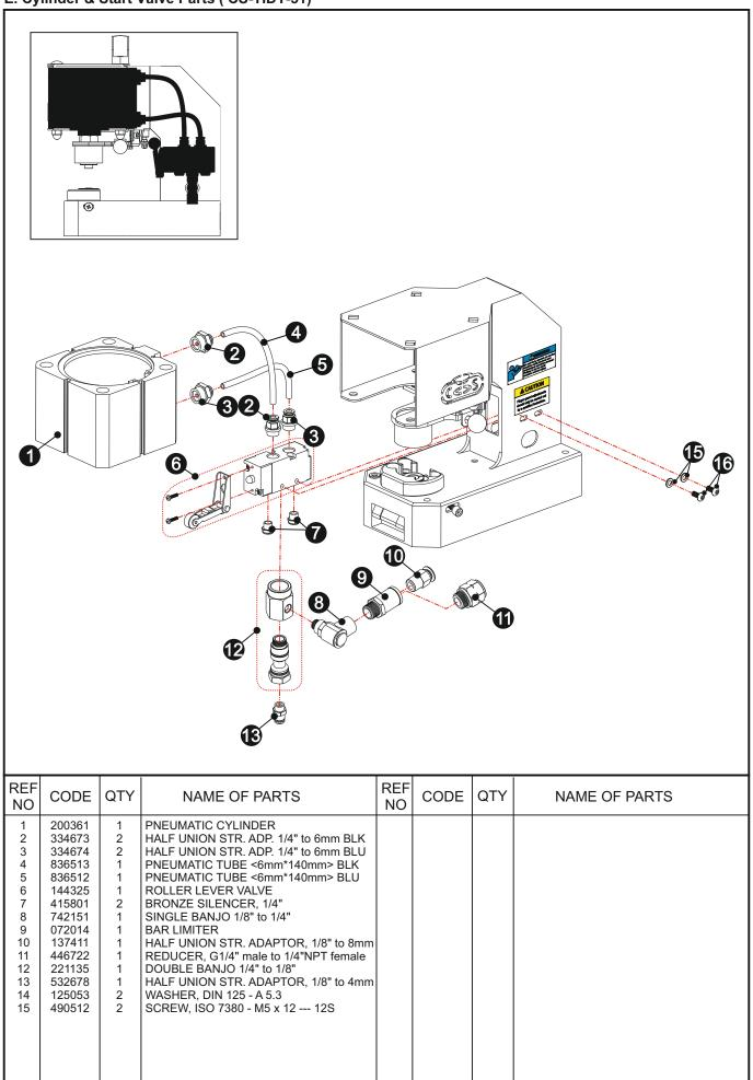
F. Safety System and Speed Controller Pneumatic Parts (CS-TIDY-51)
