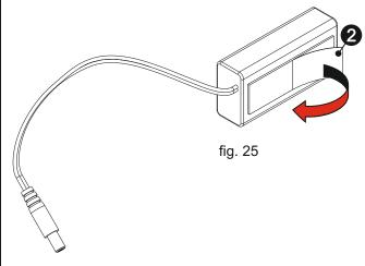
**Note:** EyeleD™ Pointer can be used with batteries or electricity adaptor. If you would like to use the EyeleD™ Pointer with the adaptor to be connected to the electricity only, you may skip following steps. Just plug in one side of the adaptor to the electricity and the jack plug to the socket at the rear of the EyeleD™ Pointer.
