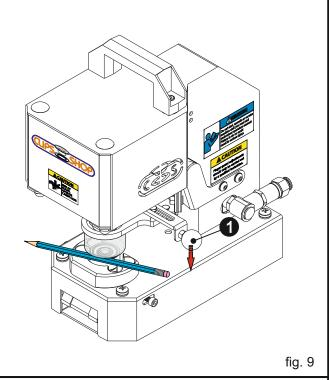
The machine should not be operated before checking the proper working of the safety guard. For testing, a test material thinner than your finger(i.e. pencil)shall be used Locate your test material (acting as your finger) as shown in the(fig.8) **Note:** Do not use a rigid test material such as screwdriver located in the middle of the die set during your safety check. You may damage the die set.
