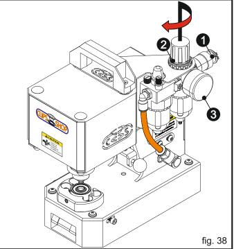
Add ISO Vg32 type oil to the lubricator. Connect your hose coming from your compressor to the slide valve ① (or to the preffered adaptor). Make sure there is air coming to the machine. Pull the head ② of the regulator upwards and adjust the air pressure coming to the system by rotating the head. You can check the pressure level from the manometer ③.
