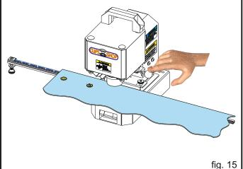
As shown in figure manually pull down the manual starting arm to operate the machine CS-TIDY-51
