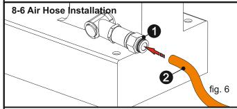
Plug in the 8 mm diameter hose coming from your compressor to the fitting for CS-TIDY-51. Turn on your air source and check the pressure in the system is averagely 6 bars. Afterwards, check if any air leakage exists.
