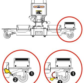
Locate the foot pedal **0** on the flap of the mobile unit **2** Install the foot pedal by fixing it with the screws **3**.
