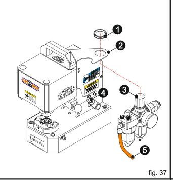
Remove the mounting nut from the regulator. Poke the regulator head through the hole on the mounting plate and fix it in position by installing the munting nut to the head of the regulator. Install the hose of the accessory to the 8 mm quick connect fitting on the air entrance of your machine. Note: You may shorten the hose as long as it is long enough to connect the air entrance of the machine with the accessory.
