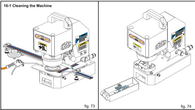
Clean your CS-TIDY-51 at least once a week with air gun. You can keep cleaning the machine with a clean cloth. **NOTE:** Do not use solvents such as kerosene or thinner to clean the machine.
