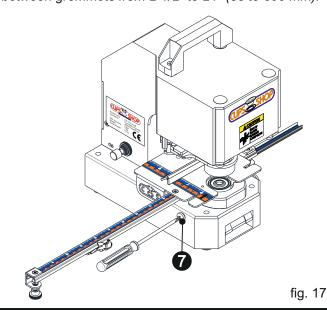
Gently tighten it manually by pushing from top. After making sure that there is no tightness or irregular connection, tighten the fixing screw with a Phillips-head screwdriver as shown in (fig.17).
