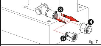
Alternatively, you can remove the 8 mm quick connect adaptor from your machine by using a suitable wrench. Then you can connect your hose that has G1/4" BSPP male adaptor to the G1/4" BSPP female adaptor part of the elbow adaptor.
