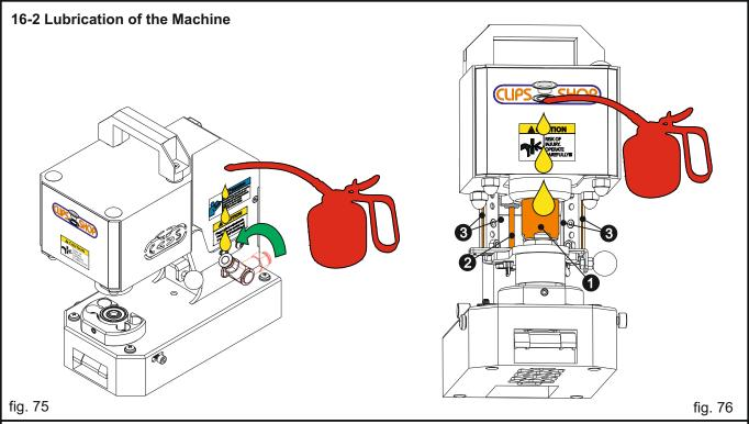
CS-TIDY-51 should be properly lubricated at least once a month. If you are using your machine frequently you shall increase the frequency of the lubrication. Before lubrication, do not forget to remove the air connection from the machine and make sure there is no air remained in the machine.
