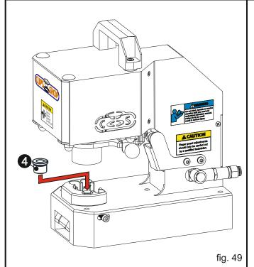
Place the lower die bush into the lower die holder by making sure its cut part faces machine's rear part.
