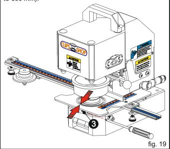
Gently tighten CSGSP-2 to the lower die holder and make sure their surfaces are at the same level. Then securely fix the screw with a Phillips-head screwdriver to secure the connection as shown in (fig. 19).
