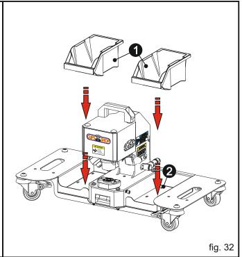
Locate the machine on the mobile stand. First poke the bolts through the washers Then poke them through the machine and the mobile stand Install the washer and nut from the bottom manually and fix the nuts with a suitable wrench.
