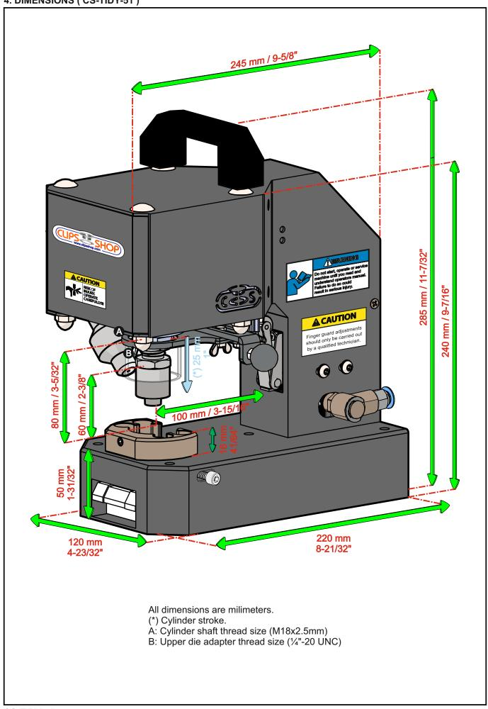
• The thickness of the table should be at least 18 mm, and it should be strong enough to bear the weight and vibration of the CS-TIDY-51 machine.
