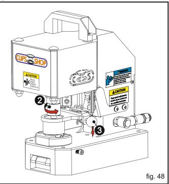
Pull down the manual starting arm to access the upper die. Securely fix the upper die to the upper die holder/shaft manually. Note:Be sure that the upper die adaptor is securely fixed to the shaft and the upper die is securely fixed to the die adaptor at all times. During a production run check that the upper die has not loosened from the die adaptor. Using the machine with a loose upper die can damage the threads of the die and the die adapter.
