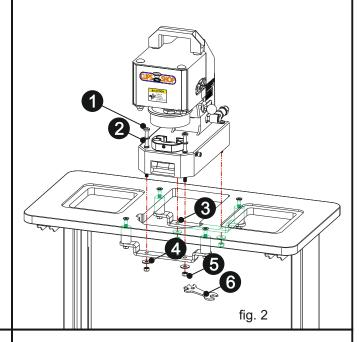
Firstly insert screws to the washers from CS-TIDY then through the head spool plates . Attach screws to the washers and nuts. Tighten the nuts with wrench for fixing.
