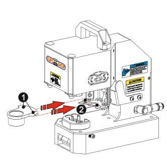
Depending on the die set you would like to use with your CS-TIDY-51, you may need to change the finger guard size. Refer to "Die Compatibility Guide" section and choose the required size of finger guard based on your grommet size accordingly die selection. The machine does not come with alternative sizes of finger guards so contact your dealer to purchase the required tools.
