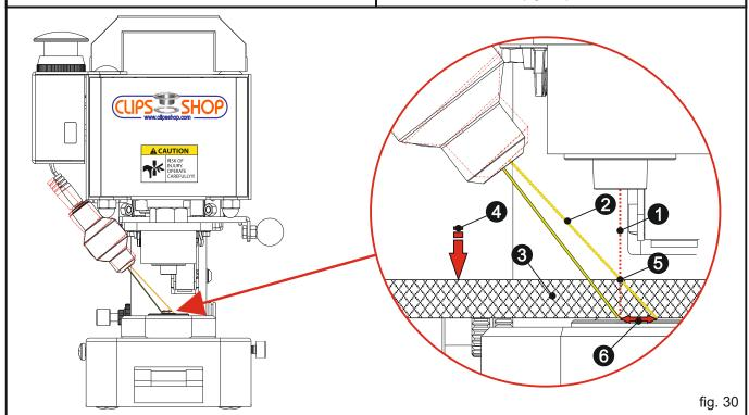
The position of EyeleD's light dot should be adjusted per the thickness of your material. This position shifts from the die center line in a distance depending on the top level of your material.
