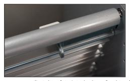
FIGURE 22 (Latch safety interlock on feed tray)
