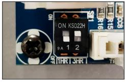
FIGURE 3 (Extended Setting: 3 Hour Standby)
