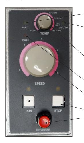
**GREEN "READY" LED** is on when roller temperature is ready. Flashes if roller temperature is too hot.
