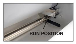
FIGURE 20 (Idle bar shown in run position)
