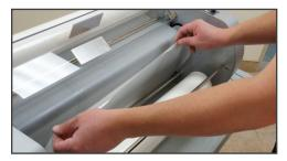
**FIGURE 17** (Apply tape to film to hold film together)
