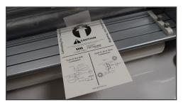
**FIGURE 23** (Threading card pushes film into nip of rollers)
