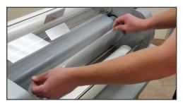
**FIGURE 16** (Pull bottom film under idle bar and drape over top film)
