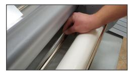
**FIGURE 15** (Slide bottom idle bar down slot to loading position)
