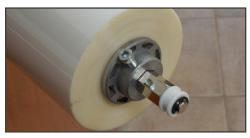
FIGURE 10 (film gripper installed)
