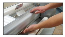
FIGURE 19 (Push idle bar to run position)
