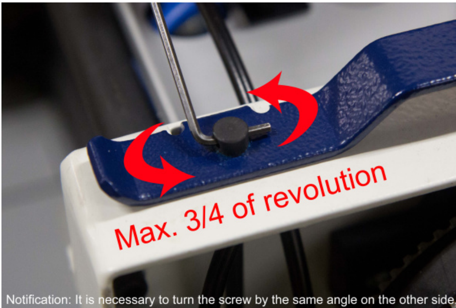
Fig. 33: Turn the fixing screw of calliper and move the shaft with feeding wheel downward. This will reduce the gap between main feeding wheel and separator.
