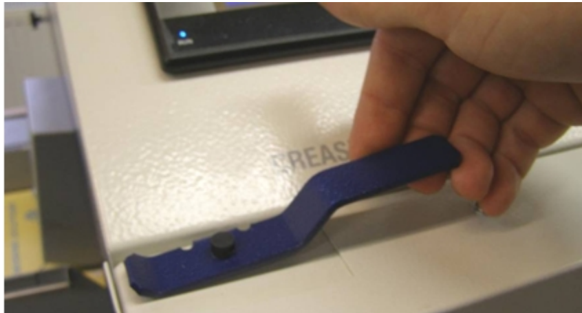
Fig. 17: Pulling callipers to the upper position
