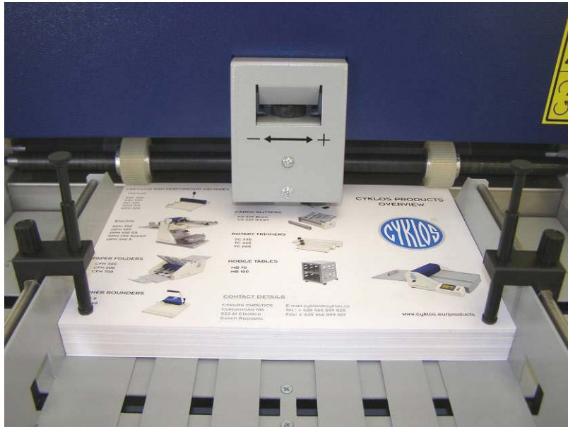
Fig. 15: Example of correct placement of paper pile
