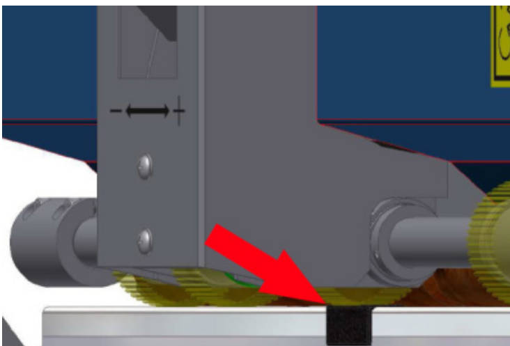
Fig. 34: The gap between feeding wheel and separator must be 0,05 – 0,1 mm wide.
