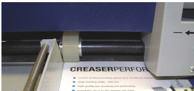
Fig. 12: Correct adjustment of the feeding wheels
