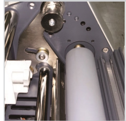
DE-CURLING BAR INSTALLED
