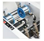
**ONE-STEP THREADING** Magnetic stitching heads feature one-step threading for quick and easy set-up.
