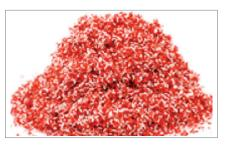
Material particle surface  $\leq 5 \text{ mm}^2$  and for regular particles: strip width  $\leq 1 \text{ mm}$  (0.8 x 5 mm particles, for example.
