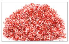
Material particle surface  $\leq 10 \text{ mm}^2$  and for regular particles: strip width  $\leq 1 \text{ mm} (0.8 \text{ x} 12 \text{ mm} \text{ particles}, for example.}$
