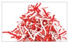
Material particle surface  $\leq$  320 mm<sup>2</sup> (4 x 80 mm particles, for example) or strip width  $\leq$  2 mm. Strip length not determined.
