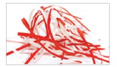
Material particle surface  $\leq 800 \text{ mm}^2 \text{ or strip width} \leq 6 \text{ mm}.$ Strip length not determined.
