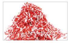
Material particle surface  $\leq 160 \text{ mm}^2$  and for regular particles: strip width  $\leq 6 \text{ mm} (4 \times 40 \text{ mm} \text{ particles}, for example).$
