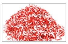
Material particle surface  $\leq$  30 mm<sup>2</sup> and for regular particles: strip width  $\leq$  2 mm (2 x 15 mm particles, for example.
