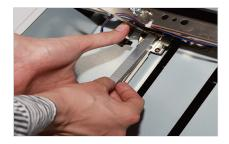
EASY STAPLE LOADING Reloading staples into a stapler magazine is quick and easy. Simply open the cover, pull the magazine, lift the plate and place staples.
