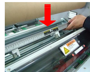
Film Slitting with Side Slitter &
