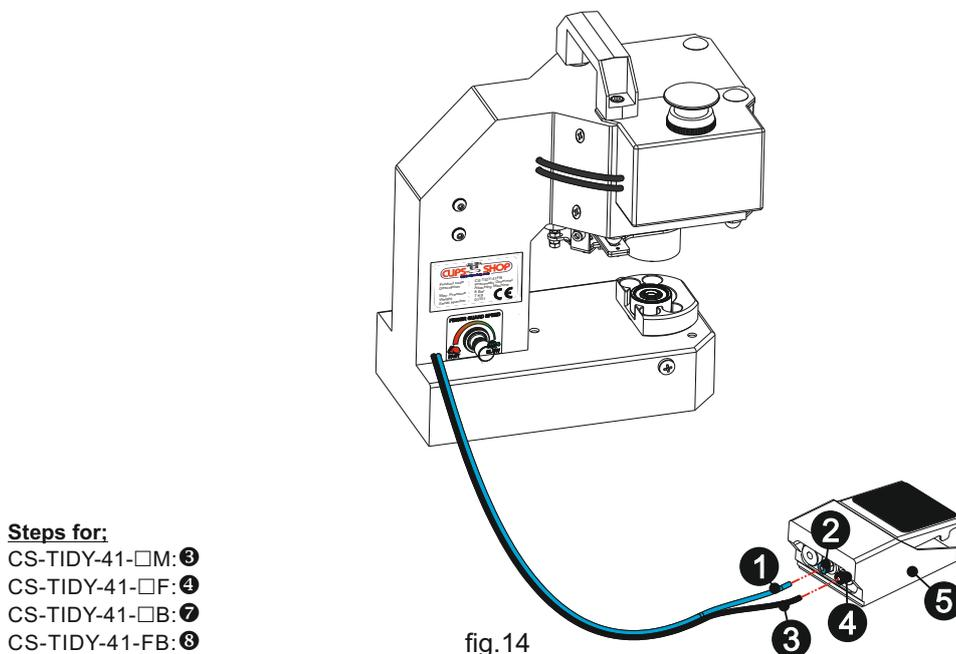
To avoid any damage during transportation, foot pedal ⑤ is packed unassembled in the factory and needs to be installed by the user.
