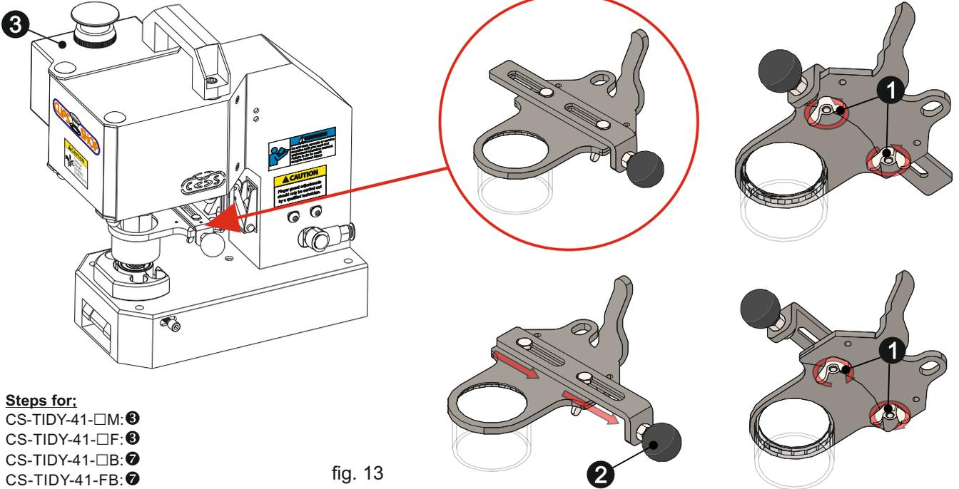
7) In order to avoid any damage during transportation, the manual starting arm ② of the machine is set to tightest position in factory settings. This arm is needed to be extended by the user for proper use. Loosen the wing nuts ① manually. Pull the manual starting arm ② in the arrow direction and adjust the length of it. Then securely fix the wing nuts ① manually as shown in (fig. 13).
