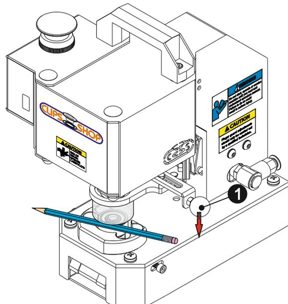
**The machine should not be operated** before checking the proper working of the safety guard. For testing, a test material thinner than your finger (i.e. pencil) shall be used. Locate your test material (acting as your finger) as shown in the (fig.17) **Note:** Do not use a rigid test material such as screwdriver located in the middle of the die set during your safety check. You may damage the die set.
