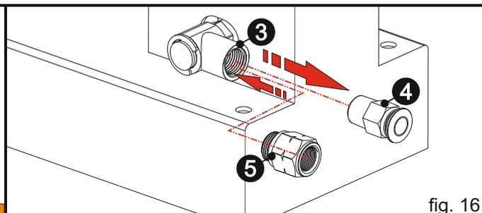
Plug in the 8 mm diameter hose<sup>2</sup> coming from your compressor to the fitting<sup>1</sup> of CS-TIDY-41. Turn on your air source and check the pressure in the system is averagely 6 bars. Afterwards, check if any air leakage exists.
