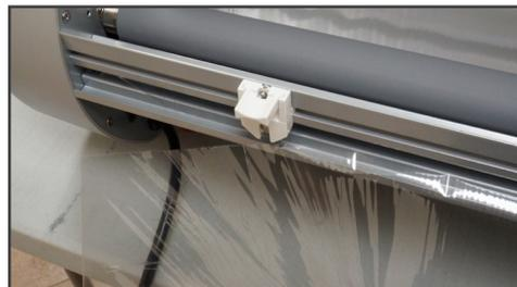
**FIGURE 27** (Film is now loaded and exiting the laminator. Wrinkles will slowly disappear as film aligns itself.)
