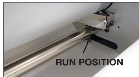
**FIGURE 20** (Idle bar shown in run position)
