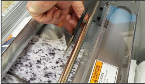
FIGURE 35 (Bottom roll film removal)
