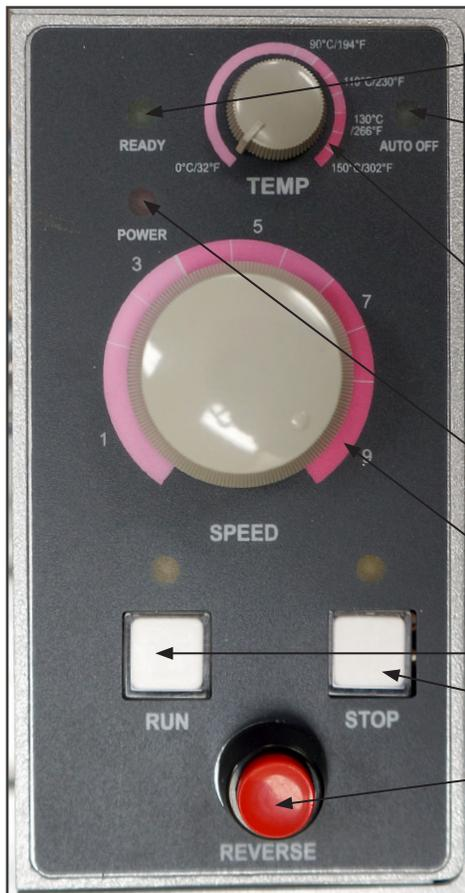
**GREEN “READY” LED** is on when roller temperature is ready. Flashes if roller temperature is too hot.
