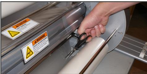
FIGURE 33 (Bottom roll film removal)
