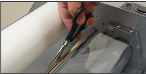
FIGURE 32 (Top roll cutting film)
