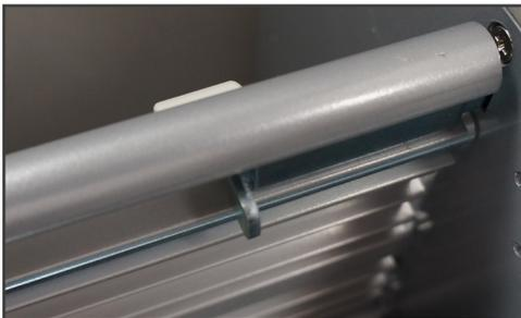
FIGURE 22 (Latch safety interlock on feed tray)
