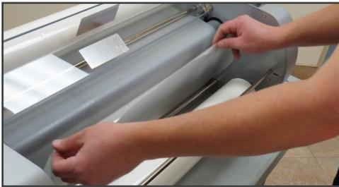
**FIGURE 16** (Pull bottom film under idle bar and drape over top film)
