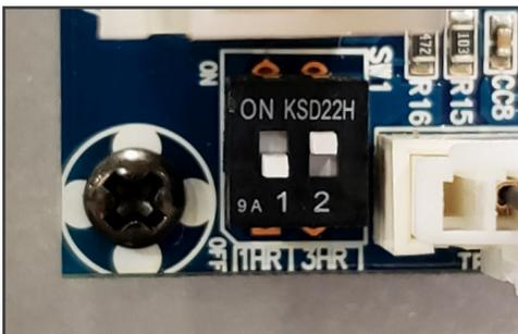
FIGURE 3 (Extended Setting: 3 Hour Standby)
