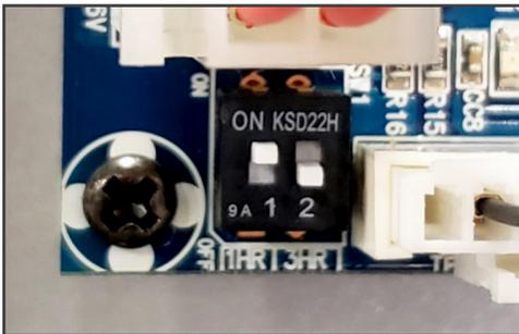
FIGURE 2 (Standard Setting: 1 Hour Standby)
