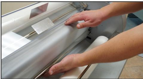
**FIGURE 19** (Push idle bar to run position)
