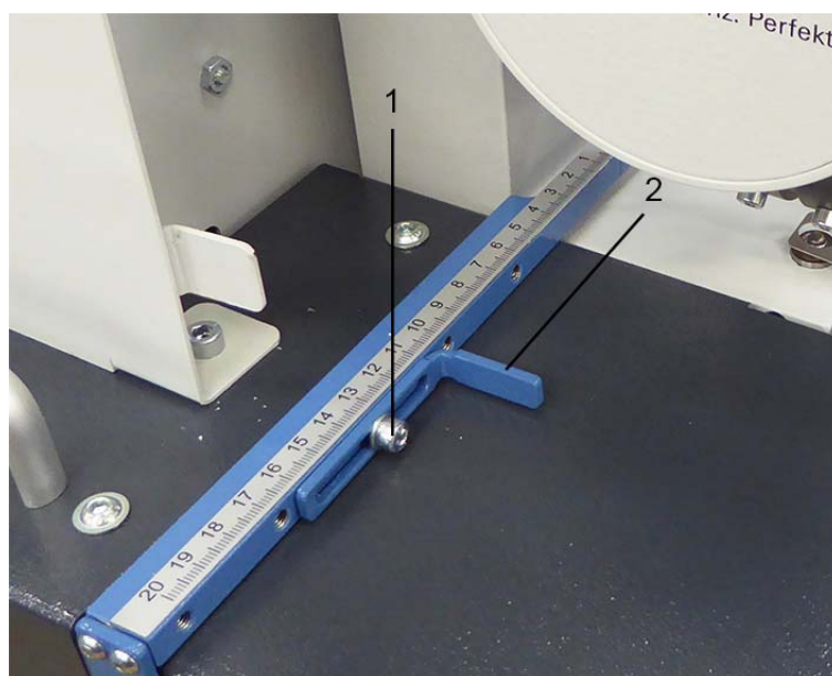
Image 6.6.2 Adjusting the lateral stop
