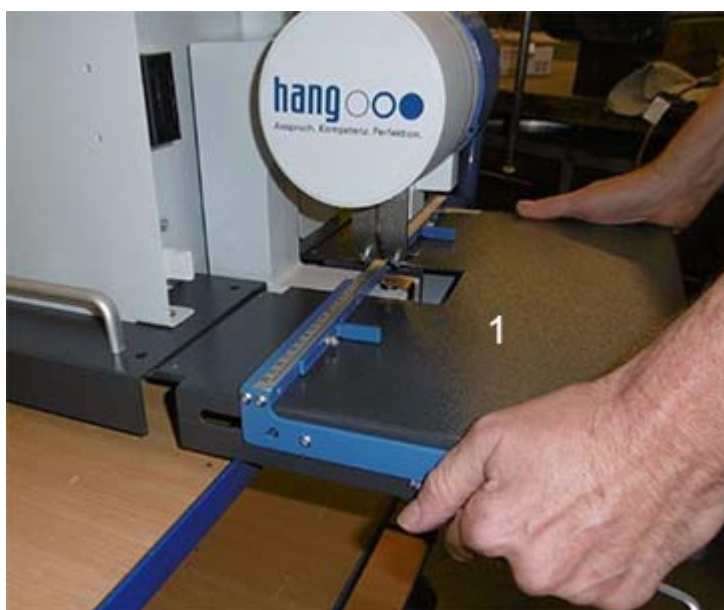
Image 9.2.2 Dismantling the lower punch
