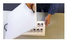
After the sheets are glued together they are placed under a **weighted board** for about 30 minutes to preventing warping.
